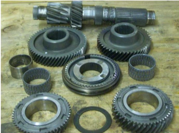
Cluster gears are pre-assembled with the big press. It takes a lot of tonnage to press 6<sup>th</sup> gear onto the cluster shaft. This photo shows the disassembled cluster.
