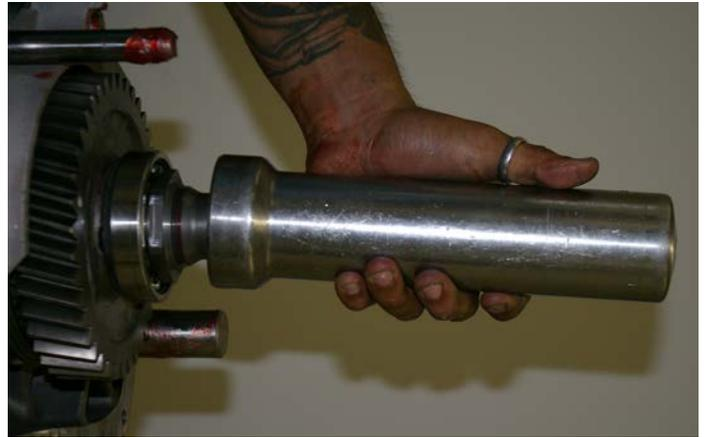
Tightening the big nut on the mainshaft with a special deep socket, to 250 ft-lb.
