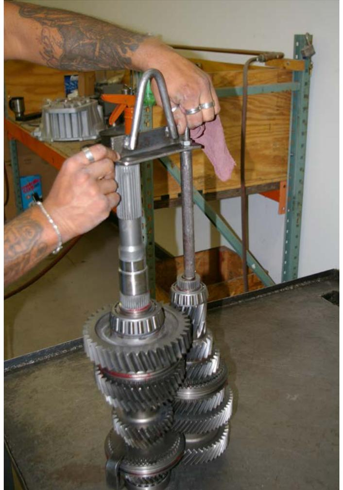
This lifting tool facilitates picking up the assembly without the components spreading apart, in order to put it into the front end of the transmission case (the bellhousing). This assembly is heavy enough that the rebuilder uses a hoist to pick it up (190 pounds).
