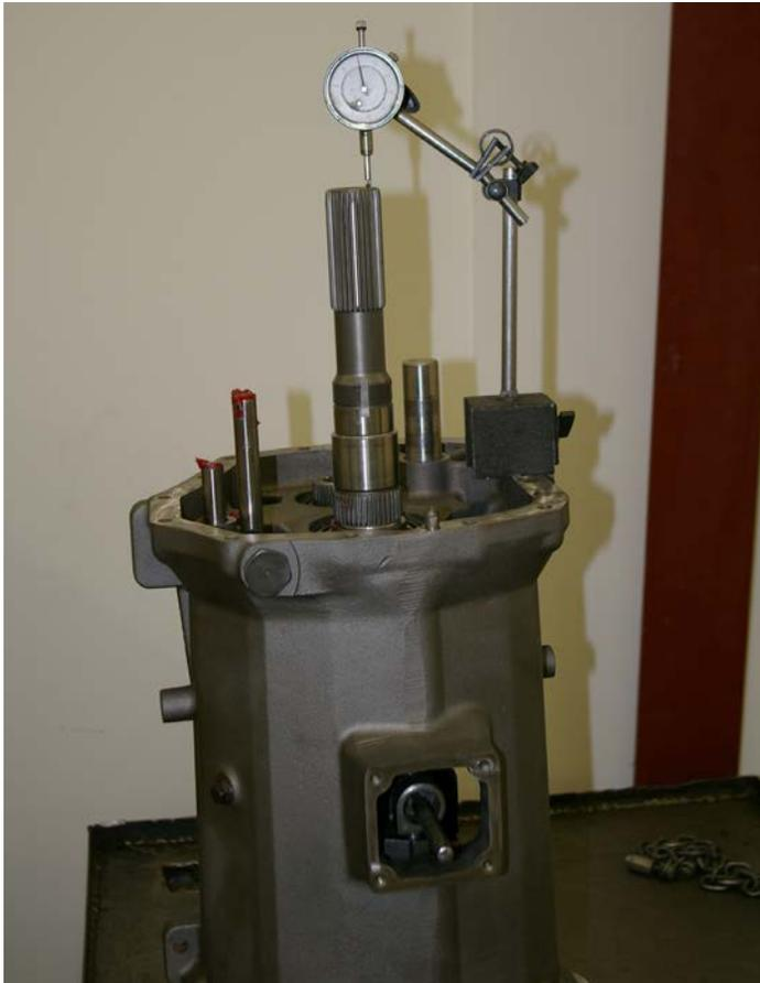
The rear of the cast iron main case, shimming the main shaft. Clearance must be checked from the rear end as shown. Shims go on the front end, under the front bearing retainer. You must turn over the partially assembled transmission to change shims each time you change them. By this point in the assembly process, the transmission weighs more than three hundred pounds.
