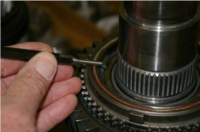
This photo shows the mainshaft turned over, starting to build the back side with first and second gear. Second gear is on, inner and outer synchronizer parts, and the friction ring are installed. The punch indicates the tab on the inner ring that has to go inside a slot in the 1,2 hub, shown in the next photo.
