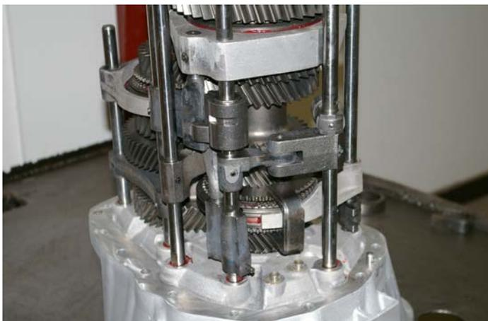
Installing the input and main gear trains, the cluster gear assembly, and the shift forks and rails. These components must all be installed simultaneously into the bellhousing/front case. This photo makes it clear that the bellhousing is far more than a simple bellhousing like the NV4500 uses. The photo shows that it is also the front plate and assembly alignment fixture for the NV5600 transmission.
