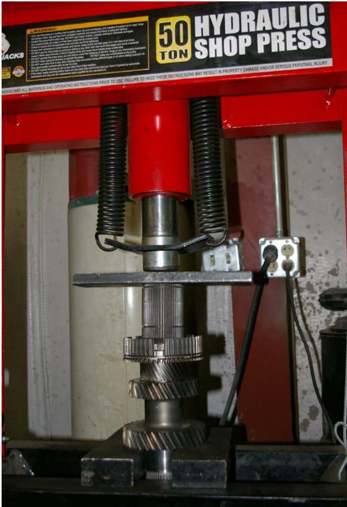
Pressing the 5-6 synchronizer hub onto the main shaft with a 50 ton press. This hub is not a light press fit. Assembly of many components requires this heavy duty press. A 20 ton press is not enough.
