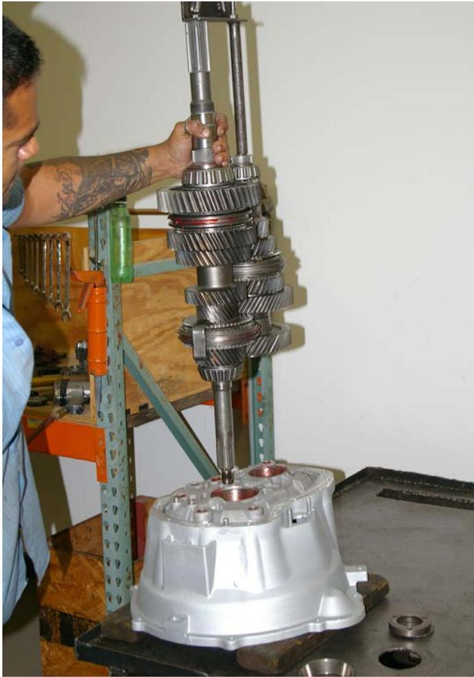
The assembly is placed into the bellhousing before the main case is installed. The main case weighs 88 pounds and the tailhousing weighs 54 pounds.
