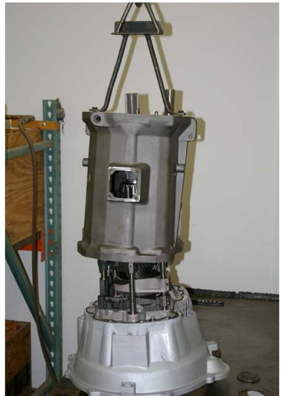
The main case is being dropped onto the bellhousing/front plate and gear train assemblies.
