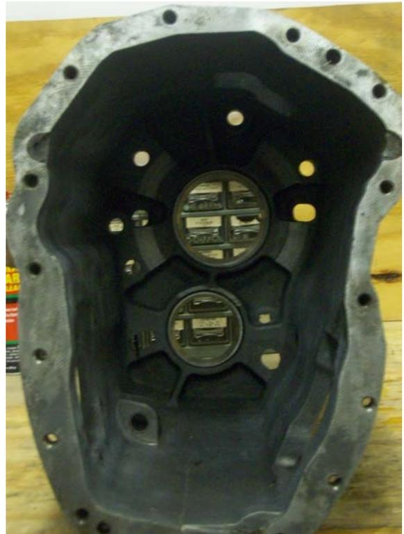
The front end of the main case. It is just an empty hole; the bellhousing/front plate is the part that retains the components.
