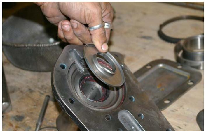
Input oil diverter in the front bearing retainer.
