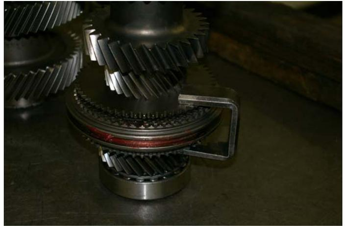
The u-shaped clamp is a trick to help put the synchronizer assembly together and keep the parts together so the balls don't spring out. The clamp shown here is being used for assembly of 5<sup>th</sup> and 6<sup>th</sup> gear, by holding the 5-6 synchronizer assembly together for installation.
