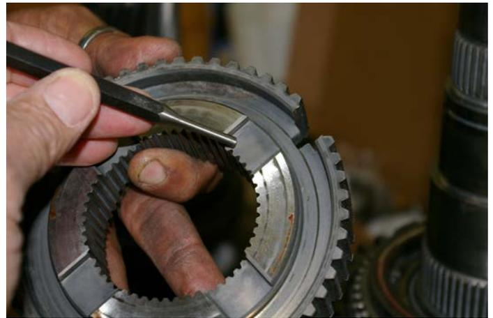
The punch indicates the notch in the hub where the tab of the inner synchronizer must go. Misalignment will result in broken tabs when the parts are pressed together.
