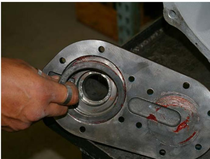
Mainshaft shim going into the front bearing retainer at the input shaft. Cluster shims are installed by an analogous procedure in the front, and checked from the rear. After shimming, put on reverse gear and install the big nut with Loctite.
