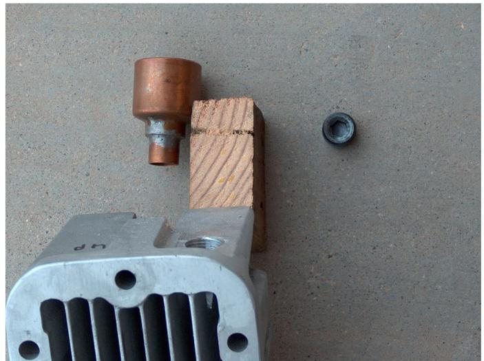
Modification to the Trans Cooler to allow filling from the top of the cooler. I used this orifice to put 6.3 quarts into my NV5600, and more could probably be poured in from there.
