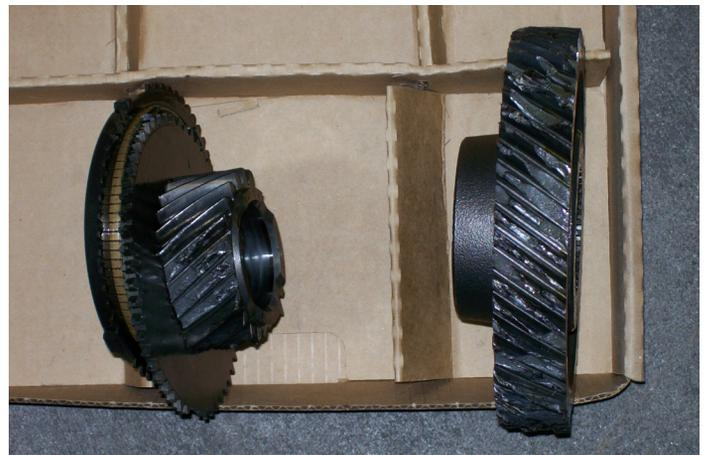
Broken sixth gears from overloading.
