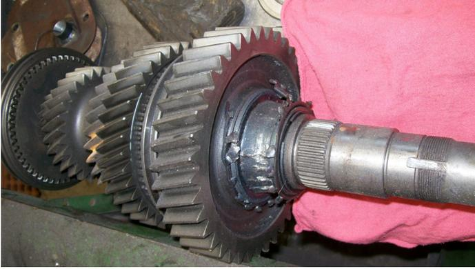
Melted first gear main shaft bearing from heavy loading, insufficient lube, and no Power Lube Package.
