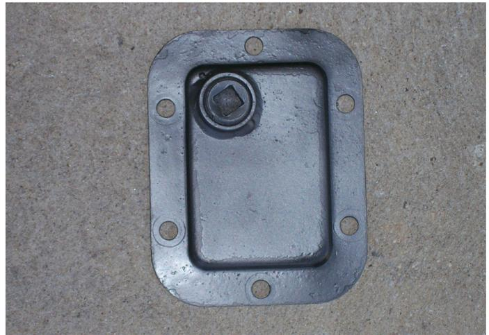
PTO cover with fill plug to facilitate adding more than four quarts of lube to the NV5600.
