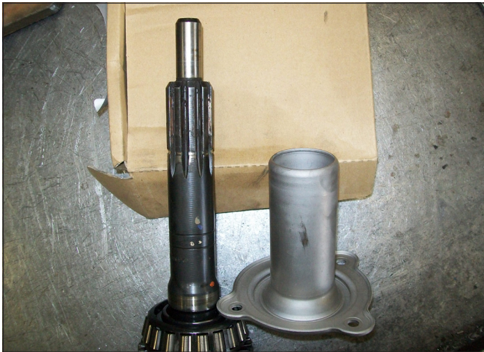
71-15 Early G56 input gear (0.79 overdrive ratio) and front bearing retainer.
