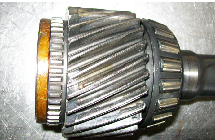
71-18 Input with wear indicating misalignment of gears.
