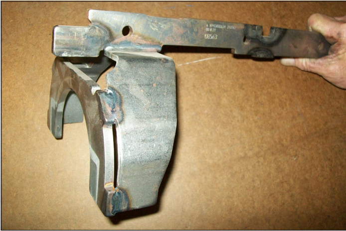
71-17 Heavy stamped steel shift fork with welds that are prone to failure.
