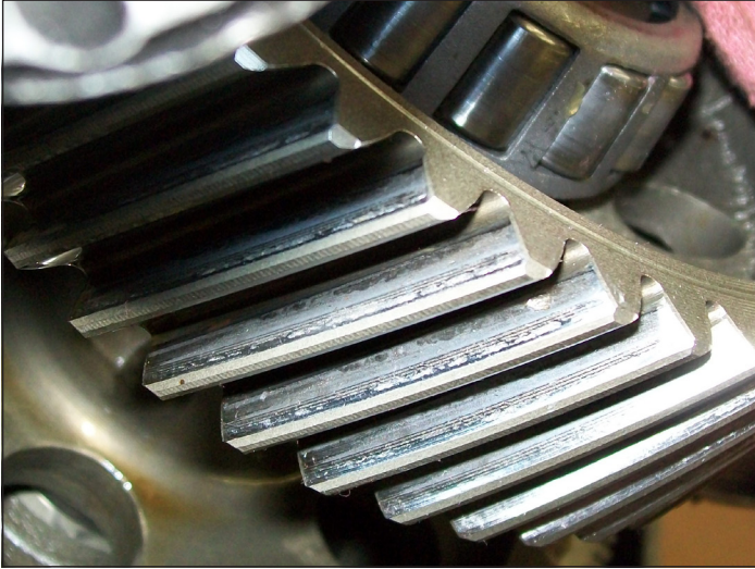
71-29 Electrolytic pitting of gear teeth.
