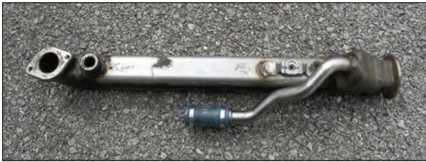
EGR cooler. Coolant enters and exits through round ports while exhaust gases enter and exit at ends.
