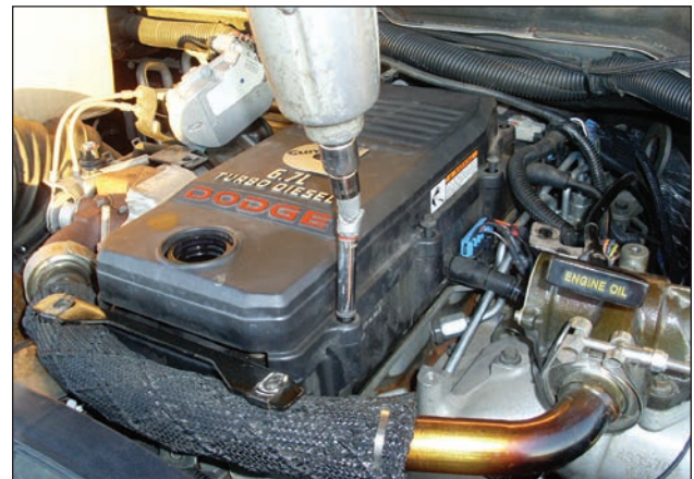
Removing the eight 8mm bolts that hold the CCV filter in place. DO NOT use the impact tool to reassemble and tighten the bolts.
