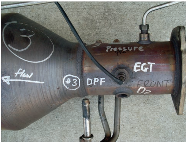
EGT, oxygen and pressure sensors monitor the need for regeneration of the NAC and DPF.
