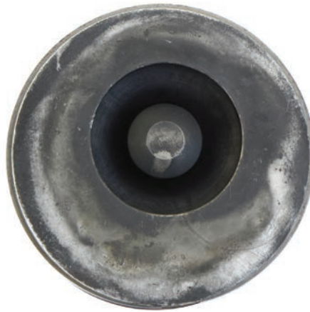
Piston top spray pattern area is visible as gray; incomplete combustion areas are black. This piston is from a vintage '94-'98 12-valve engine. Notice that the piston bowl is offset. The reason for this is that the injectors on 12-valve engines came into the cylinder head at an angle. On 24-valve engines ('98.5-'02) and HPCR engines ('03-current) the piston bowl is centered to match-up with the injector that comes into the cylinder head from directly above.
