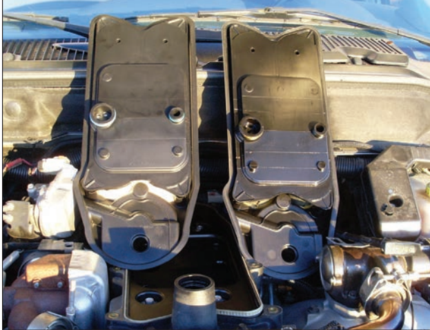
New CCV filter on the left. At 30,000 miles the CCV filter on the right looked clean and was reinstalled.
