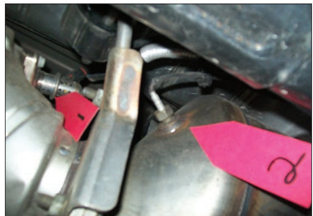
Arrow #1, DEF dosing valve. Arrow #2, EGT3 sensor
