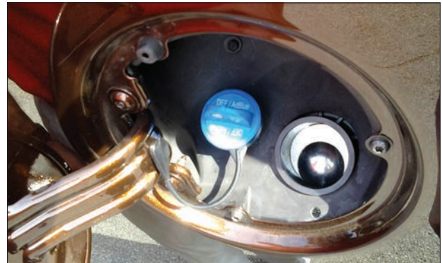
Fill DEF on the left, diesel fuel on the right.
