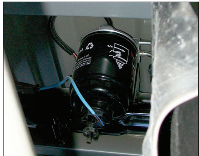
The new under-bed fuel filter.
