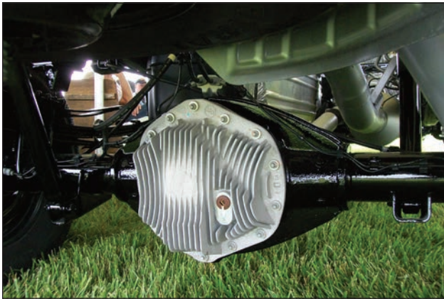
11.8" (300 mm) ring-gear American Axle differential with finned aluminum cover, for the Cummins/Aisin/dually application.
