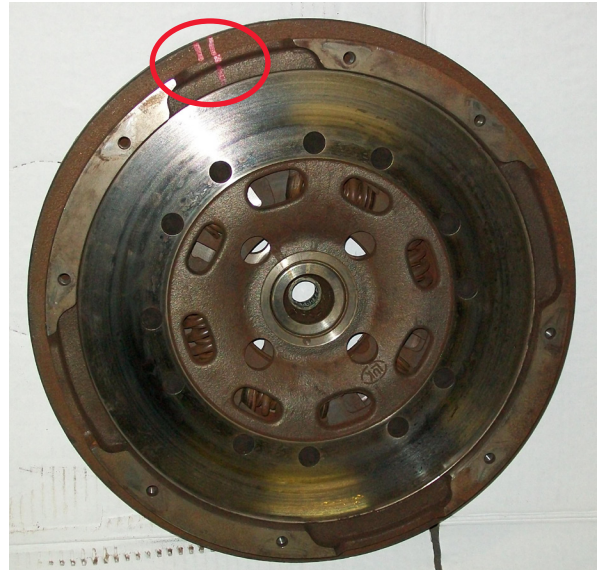
D. This close-up view of the dual mass flywheel shows that there is more than a half-inch of rotational free play.
