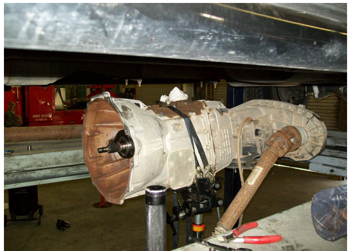
F. G56 transmission and transfer case ready for reinstallation.
