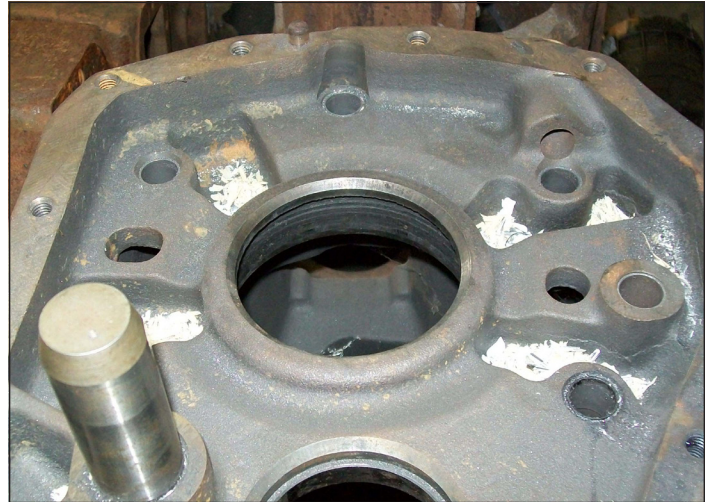
71-2 NV5600 main case with worn hole for main shaft bearing in the middle of the photo.
