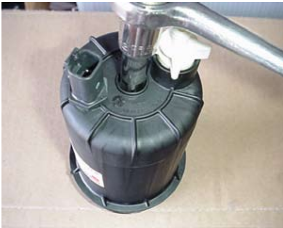
I'll bet you didn't know that there was a 1/2" drive indentation on the bottom of the filter canister.
