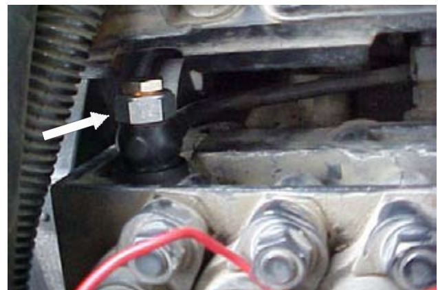
The Bosch P7100 over-flow valve.
