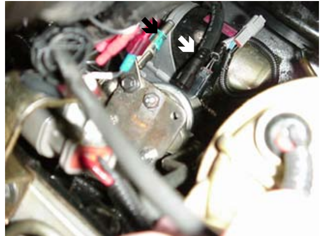
The fuel line to the transfer pump and the fuel line that goes to the fuel tank are pictured here.
