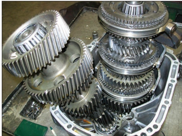
71-27 Separation of cluster and mainshaft assemblies after moving reverse idler gear out of the way.
