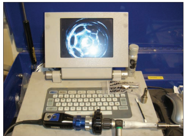
72i8. Borescope on-screen view of the inside of an extrude honed 12-valve injector nozzle.
