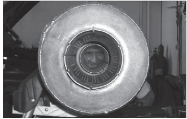
Here is Doug looking through the 4" diameter Nelson muffler, showing the straight through geometry of the 51" long internal piping. Even the analytics among us lighten up once in a while . . .
