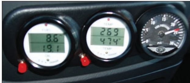
Gauge cluster installed on the test truck, capturing several parameters while the vehicle was moving. Not shown is an SPA pre-turbo EGT and boost gauge.
