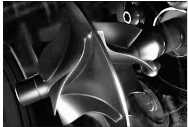
The Dual Boost turbo has a set of blades on each side of the compressor wheel, each set spinning in its own inlet housing, but feeding air to the same outlet housing.
