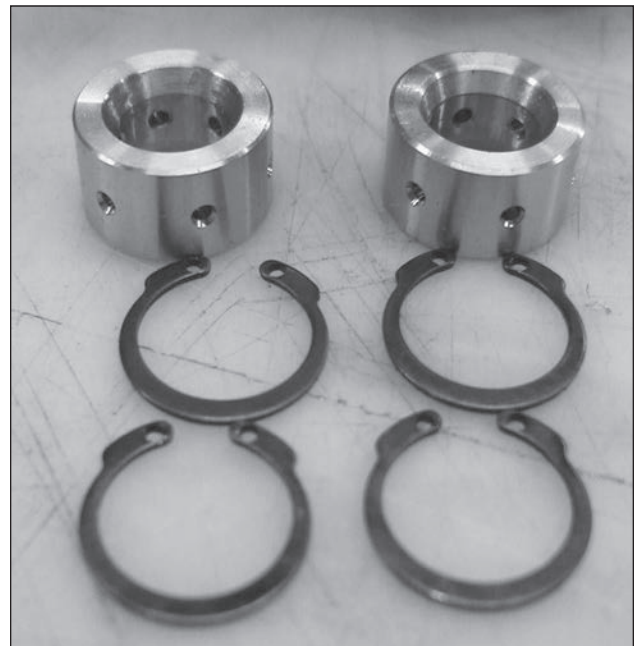
Figure 3: More robust bearing structure of the Aurora 2000. The bearings are held in place with snap rings which allows precision placement in the cartridge. The bearings rotate with respect to the cartridge and independently from the shaft, and see only about half of the actual shaft rpm.
