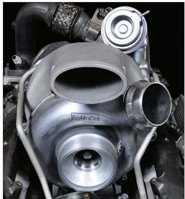
The upper and lower openings are both compressor inlets, the tube pointing to the right sends the output of both compressor wheels to the intercooler.
