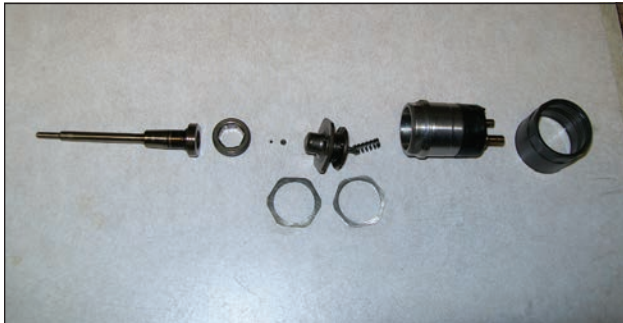
72i17. Disassembled top half of HPCR injector.
