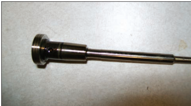
72i18. HPCR injector armature showing built up sludge.
