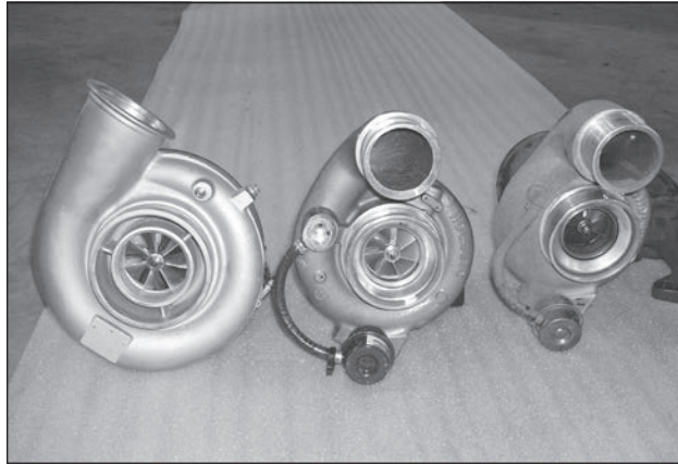
The very large ATS Aurora 5000, left, shown next to the stock turbocharger supplied for the '04.5-'05 trucks (center) and for the '03-'04 trucks (far right). The Aurora 5000 compressor loves high engine rpm, spools very aggressively starting from about 10-15 psi, and easily achieves 50+ psi.
