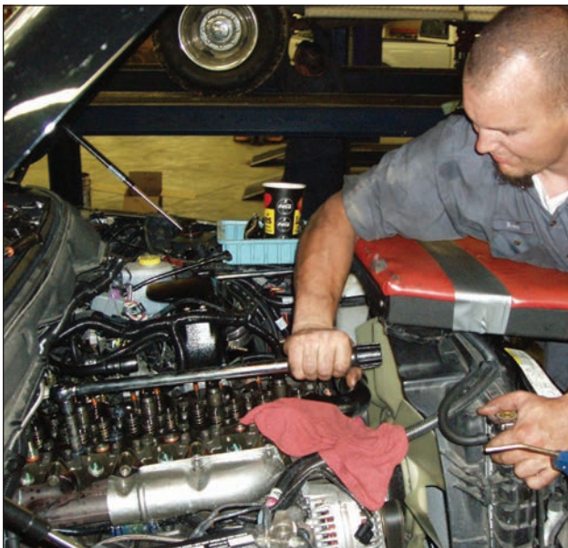
ATS mechanic Eric Daffery installing ARP head studs on the test truck. The studs are each torqued three separate times, at 70, 100, and finally 125 ft-lbs. See "TDRRelease," in TDR Issue 45, page 156, for the vendor product announcement.
