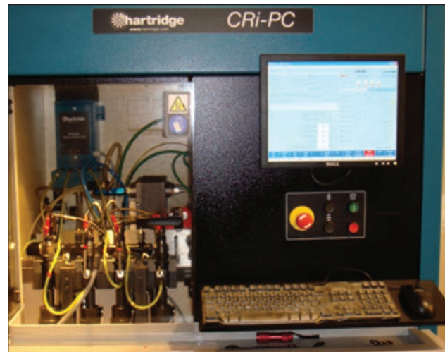
Hartridge injector tester to determine leakage, flow rate, and response time.
