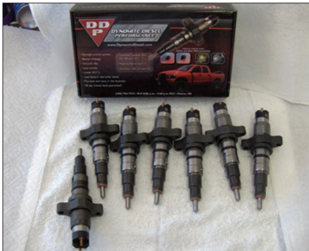
Six new DDP Stage 1 injectors with shiny white stainless steel bodies; and facing the other way is a used injector with the regular gray colored steel body.
