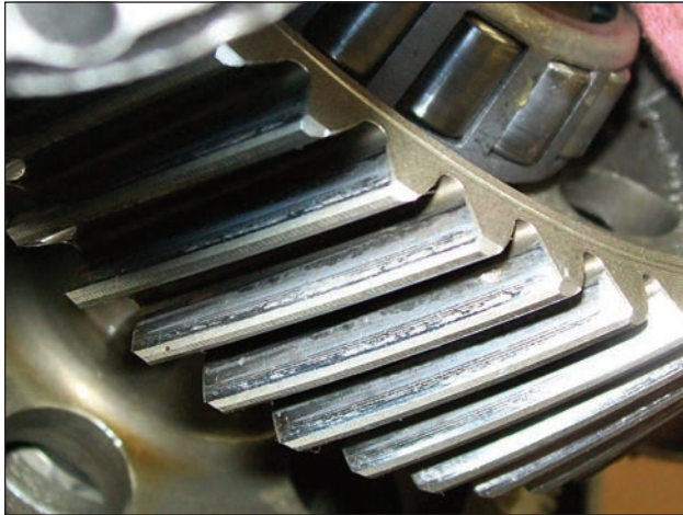
71-29 Electrolytic pitting of gear teeth.
