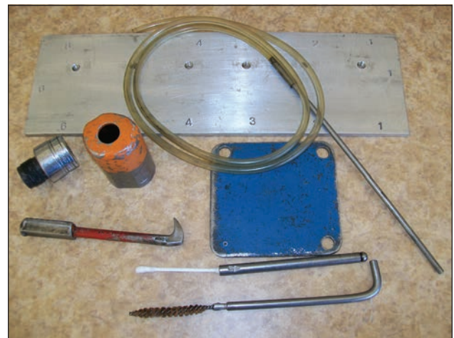
72i20. Specialty tools for HPCR injector replacement.
