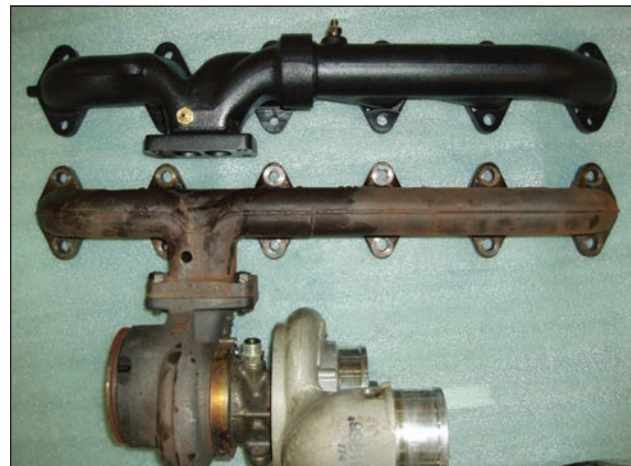
ATS two-piece manifold (top). Note the more robust design, and the expansion joint (arrow) which prevents cracking when large power enhancements are used.
