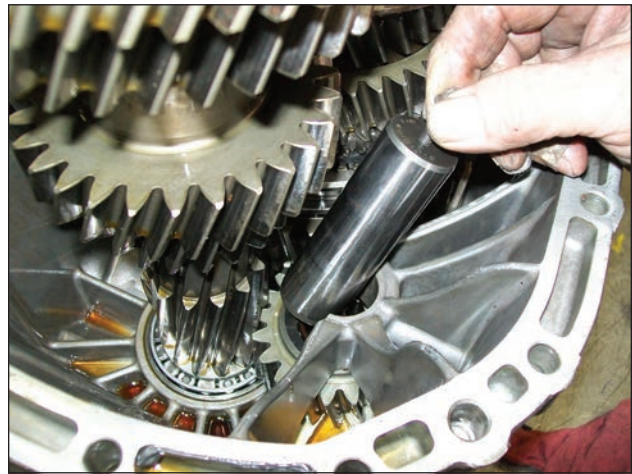
71-26 Removal of idler gear shaft.
