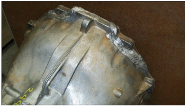
71-23 Welded but distorted G56 case at bell housing area.
