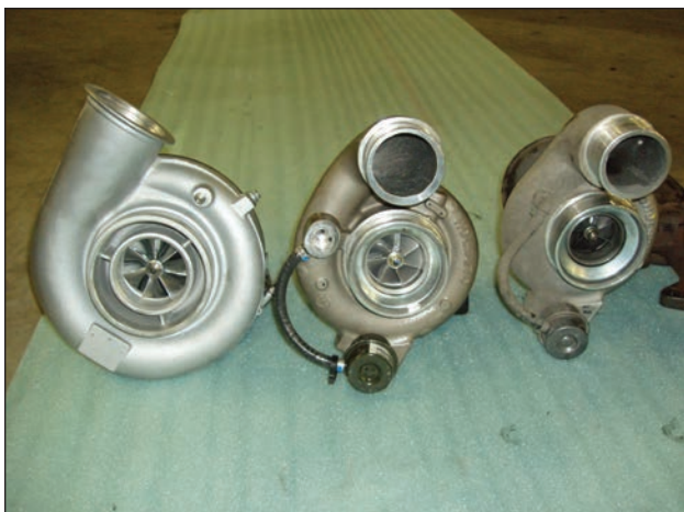
The ATS Aurora 5000, left, shown next to the stock turbocharger supplied for the '04.5-'05 trucks (center) and for the '03-'04 trucks (far right). The very large Aurora compressor loves high engine rpm, spools very aggressively starting from about 10-15 psi, and easily achieves 50+ psi.
