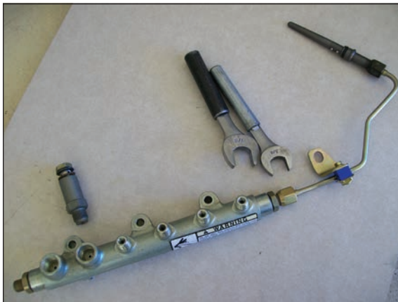
72i4. The high pressure fuel rail with the pressure relief valve above it on the left. In the center are the shortened wrenches used to remove the #6 fuel line while clearing the cowl of the truck. The #6 line is threaded into the rail and an injector connector tube.
