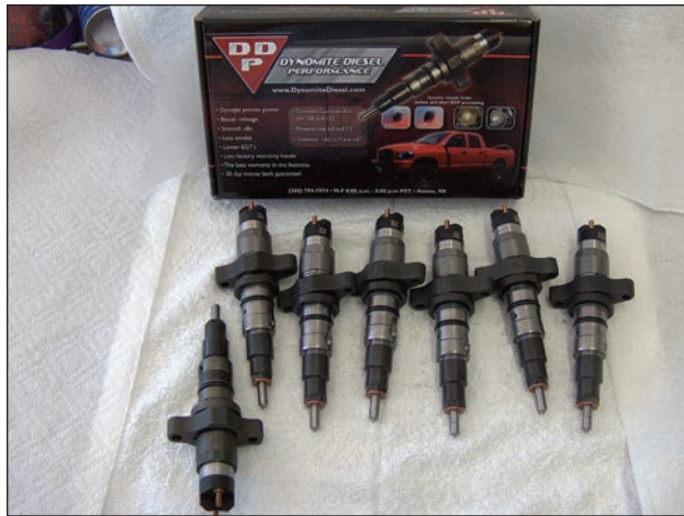
72i11. Six new DDP Stage 1 injectors with the new Bosch shiny white coated steel bodies. Facing the other way is a used injector with the regular grey colored steel body.
