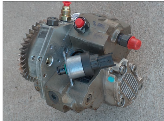
72i1. The rear of the Bosch CP3 high pressure pump showing the finned cover of the gear type pump at lower right. The Fuel Control Actuator is lying on the pump and attaches on the rear left side of the pump.
