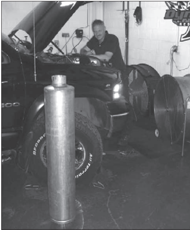
The 51" long Nelson 86131 muffler, affectionately referred to as "the water heater" by TDR member "100 Proof," Michael Keys, who generously helped during the installation. Don Bentley, owner of Meridian Motorsports, looks on in the background. Don operated the Dynojet 248 for all of the new experimental runs used in this article.
