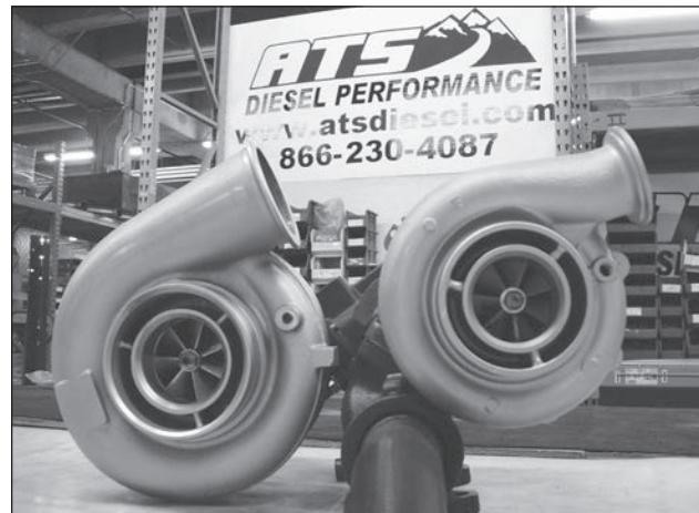
The ATS Aurora 2000 small single, right, shown next to the Aurora 5000 large single, left. Note the smaller compressor housing of the Aurora 2000, used to achieve fast spool-up. The Aurora 2000 is useful for power levels up to approximately 450 horsepower at the rear wheels.
