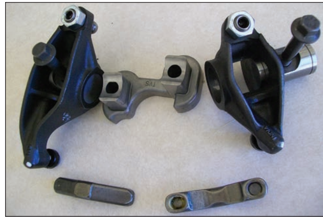
72i21. Rocker assembly for one cylinder. Exhaust, pedestal, intake, rocker pivot shaft and bolt, and two bridges below to couple pairs of intake or exhaust valves.
