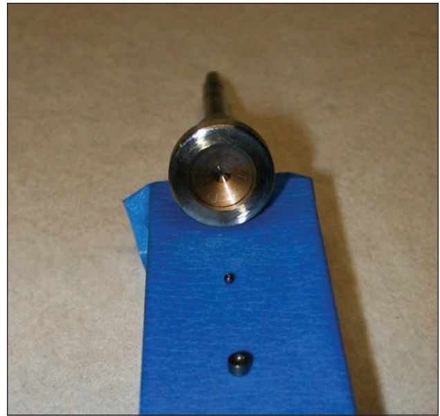
72i19. Fuel return seat, check ball, and end of armature.
