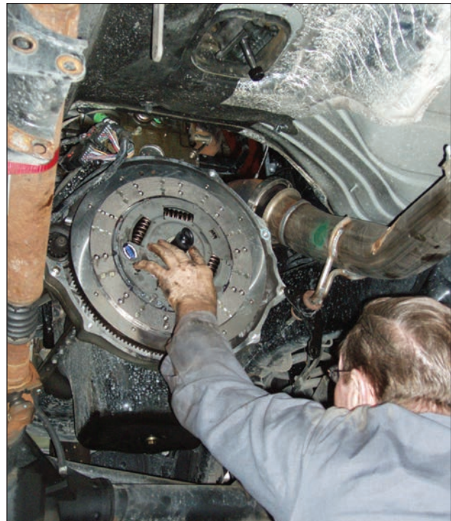
ATS mechanic Joe Johnson installing the South Bend Con-FE clutch. The disconnected front drive shaft is visible on the left, and the exhaust downpipe is visible on the right.
