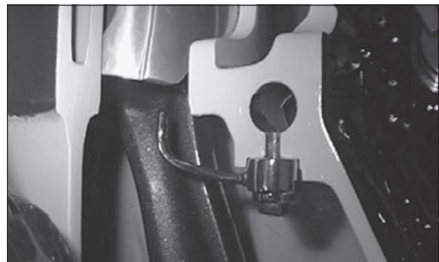
The J-jet piston cooling nozzle.
