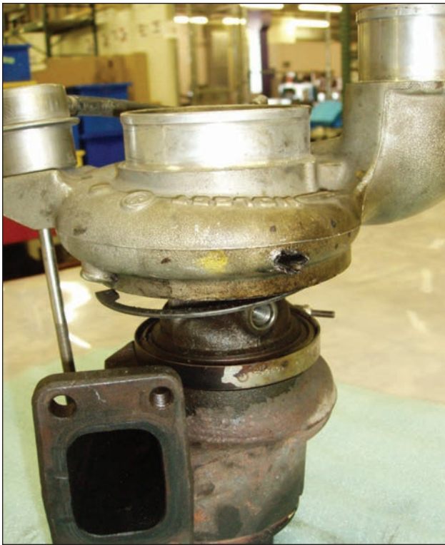
Stock HY-35 turbocharger (from an '03-'04 truck) that was destroyed from the use of aggressive fueling enhancements. The compressor wheel literally flew apart and broke through the compressor housing.
