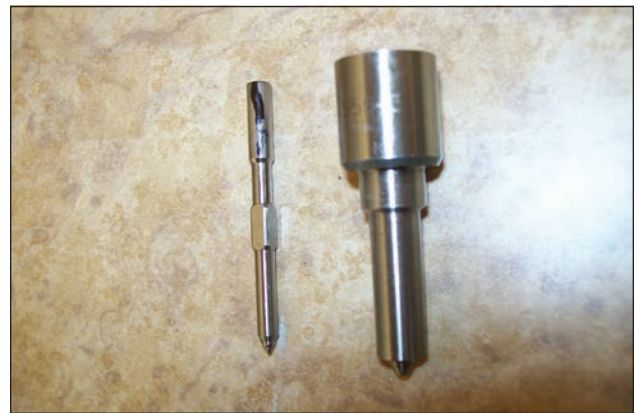
72i12. Pintle with Magic Marker stripe, showing inadequate clearance for the nozzle.
