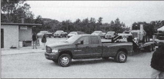
This picture shows the three trucks set up for the towing test. Each loaded trailer weighs 13,000 pounds and is mounted to the truck with a gooseneck hitch.
