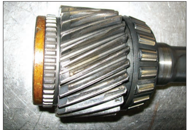
71-18 Input with wear indicating misalignment of gears.
