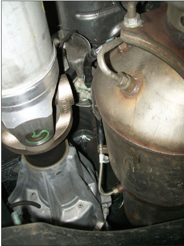
12. Pressure sensors before and after the DPF, with electronic module above them (in the photo, partially hidden behind the driveshaft universal joint).
