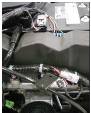
In the previous engine there were individual noise isolators attached to the fuel injection lines (left picture). Now there is a rubber isolation boot that covers the injection lines (right).
