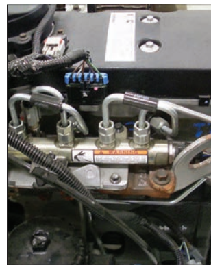
In the previous engine there were individual noise isolators attached to the fuel injection lines (left picture). Now there is a rubber isolation boot that covers the injection lines (right).
