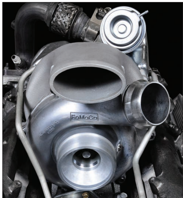
The upper and lower openings are both compressor inlets, the tube pointing to the right sends the output of both compressor wheels to the intercooler.
