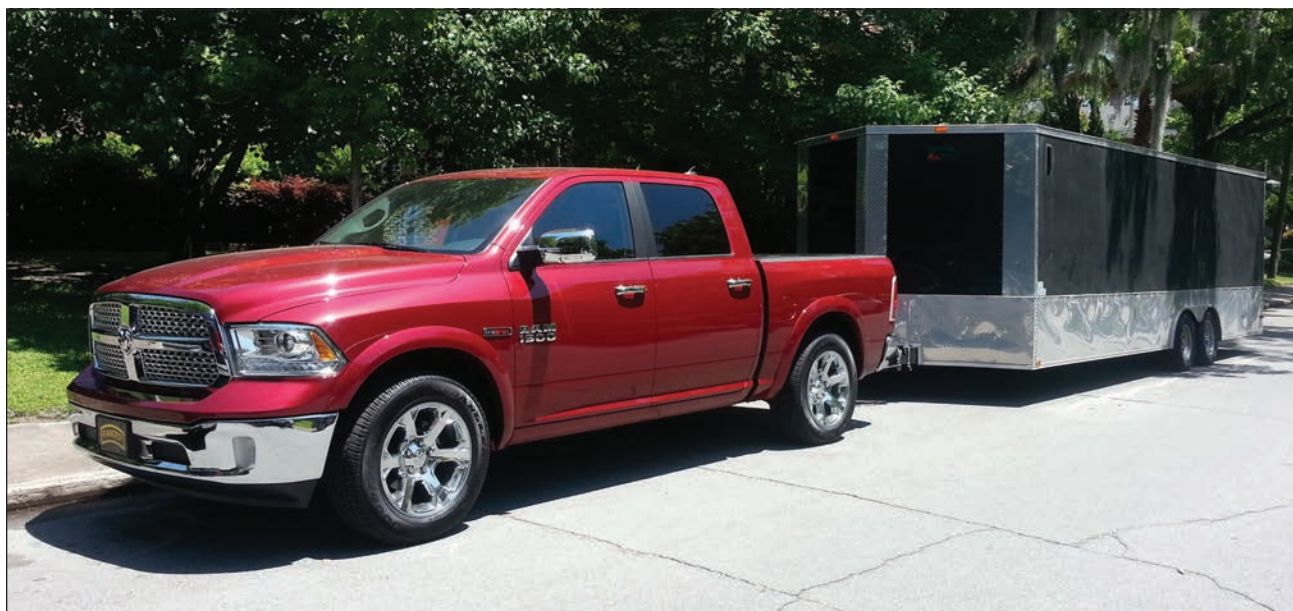
With a 24', 7400 pound trailer, 800 pounds of tongue weight and 200 pounds in the bed, the airbags keep the truck level.
