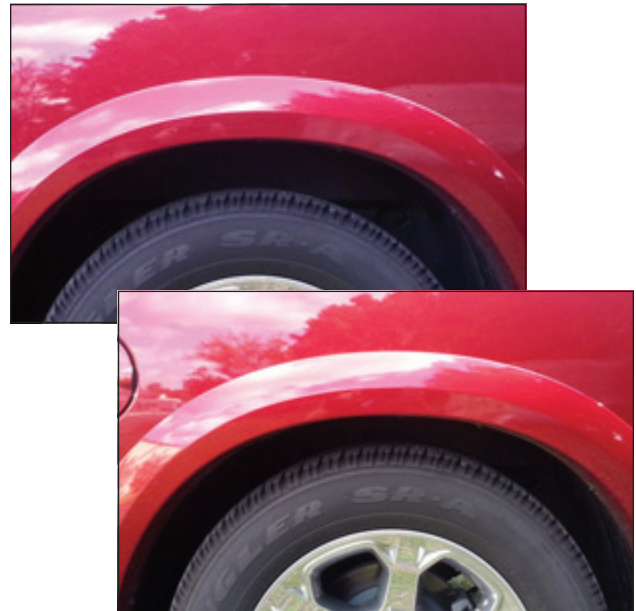
Before with 1 in sag (top) and After with 3 in. sag (bottom).
