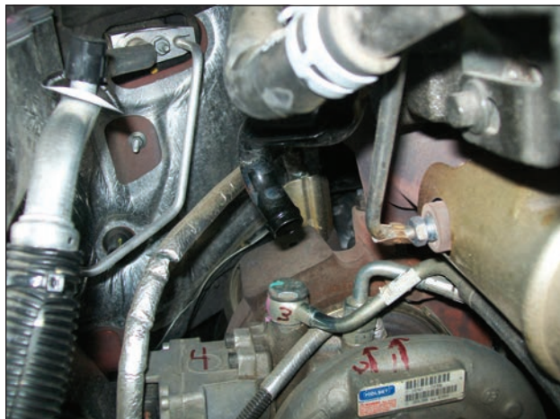
Arrow #1, turbocharger speed sensor under the foil cover for the wiring harness.
