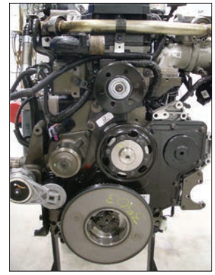
Higher horsepower, more heat, more cooling is necessary. The old engine is on the left, new on the right. Study the photographs carefully and you should see that the water pump and fan drive pulleys are slightly smaller so that they spin faster to provide better cooling.
