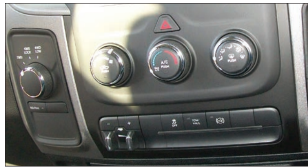
Knob for electric shift transfer case, HVAC knobs to the right of it. The switch panel is below, with the trailer brake controller at the left, and the Tow/Haul mode switch in the center.
