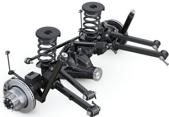
2500 Ram rear coil suspension.
