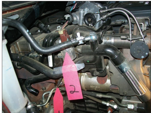
Arrow #1, exhaust gas pressure tube and fitting in the exhaust manifold. Arrow #2, electronic sensor for pressure readings.
