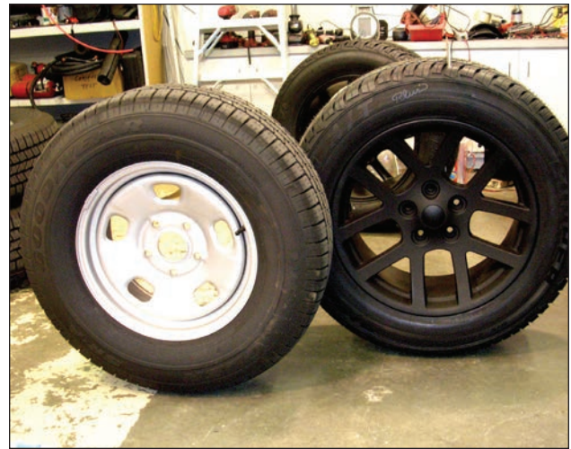
Yes, total diameter of the tire changes the overall gear ratio. Even though the 20" wheel/tire combo is in the background, you can still see that it is taller than the stock wheel/tire combo.
