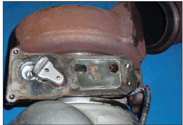
The gear rack on the left connects to the linkage that moves the vane sleeve. The two holes to the right of the gear are coolant passages.
