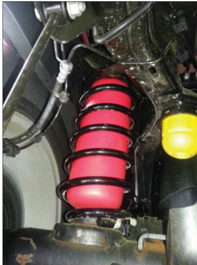
Airlift 1000 airbag, a must do for serious loads in the bed. $90 and a one hour install.
