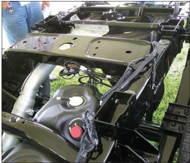
Frame showing welded pockets on the top of the rail for fifth-wheel hitch mounts, and the cross member that the gooseneck hitch mount bolts to, on the underside of the member.
