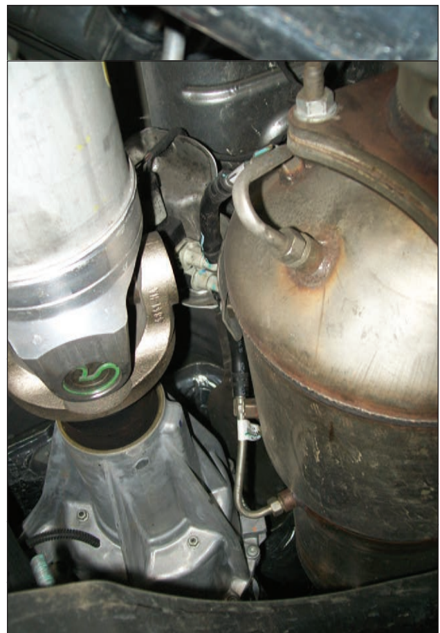
12. Pressure sensors before and after the DPF, with electronic module above them (in the photo, partially hidden behind the driveshaft universal joint).
