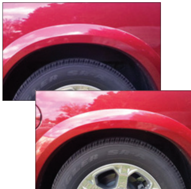
Before with 1 in sag (top) and After with 3 in. sag (bottom).
