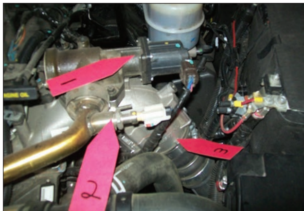
Arrow #1 EGR flow control valve. Arrow #2, EGR temperature sensor. Arrow #3, intake air throttle valve with the controller shown to the right of Arrow 2.
