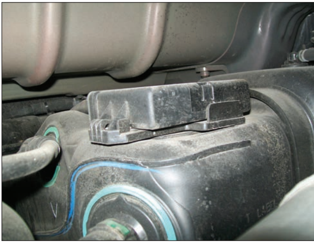
13. Dosing control module on top of the DEF tank.
