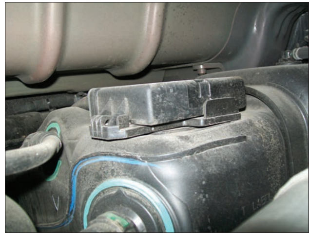
13. Dosing control module on top of the DEF tank.
