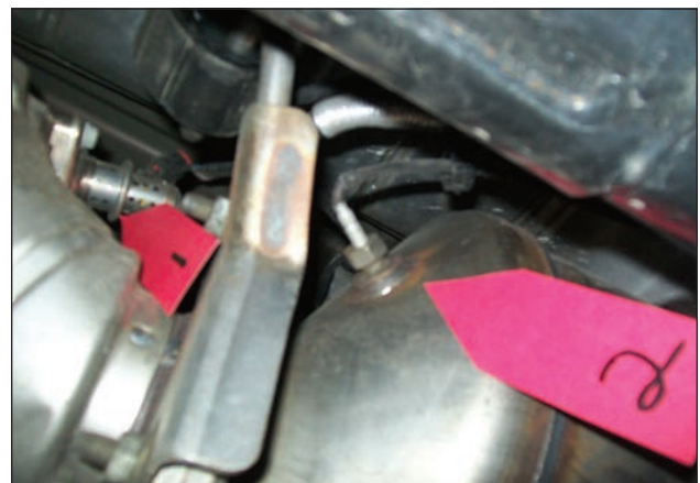
Arrow #1, DEF dosing valve. Arrow #2, EGT3 sensor
