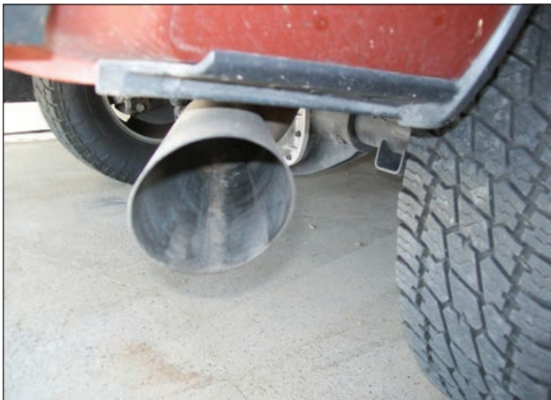
Ram Turbo Diesel tailpipe after 40,000 miles.
