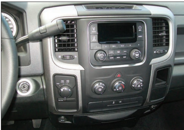
Uconnect 3.0, HVAC knobs underneath the screen, electric transfer case switch to the left of the knobs, and ignition switch to the left of that, just right of the steering wheel.
