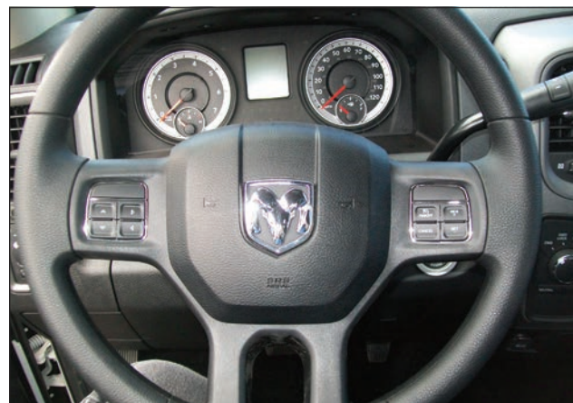
ST steering wheel and standard instrument cluster, with EVIC display screen in the center of the cluster.
