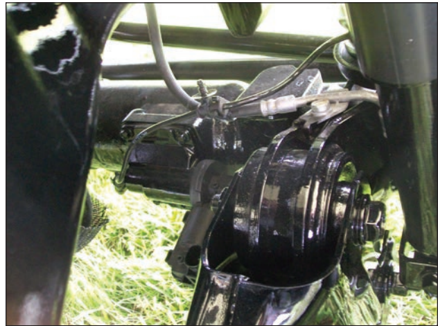
Front axle disconnect is to the left of the suspension arm pivot and under the brake hose.
