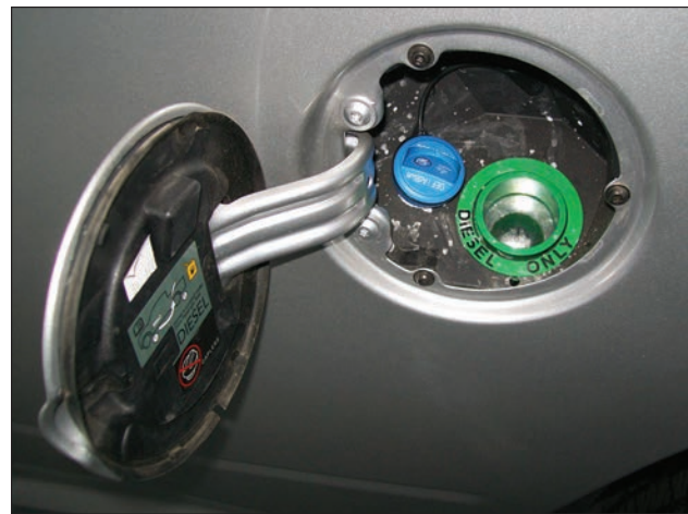
Open fuel door, showing DEF and diesel fuel inlets.
