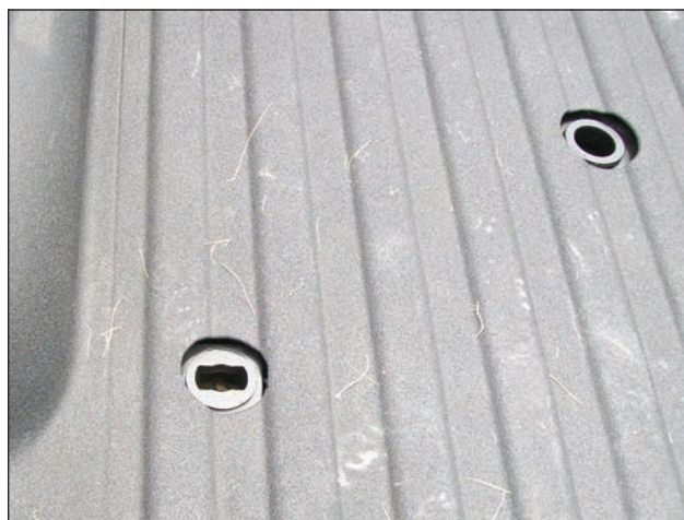
One fifth-wheel mount pocket in the bed at the lower left, and the gooseneck ball mount in the upper right.
