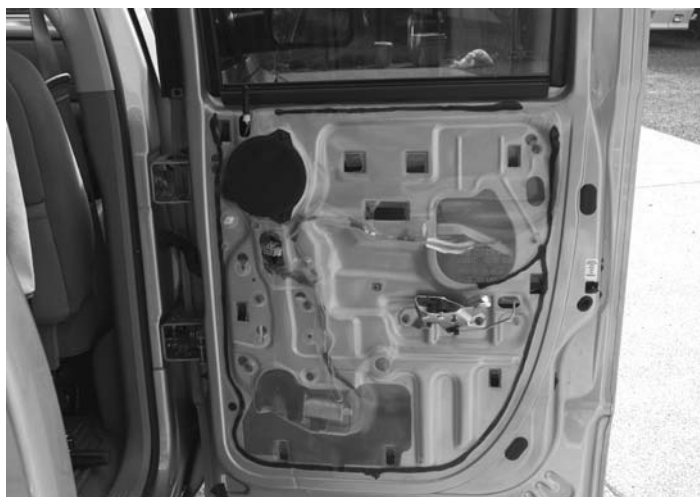
We upgraded the sound control in our '05 Turbo Diesel with the use of Dynamat. Pictured are doors and rear cab wall before Dynamat.
