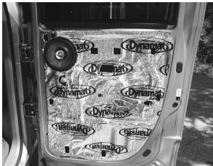
We unplugged the factory speakers and used the adapters provided by Crutchfield. The new Infinity Reference 6021 speakers fit nicely using the mounting hardware provided.
