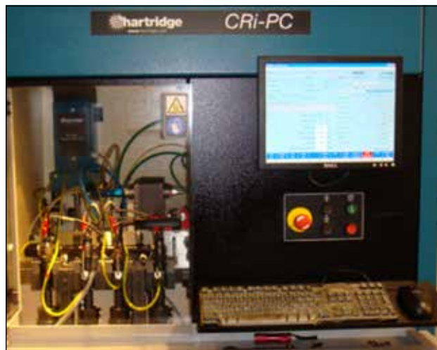
Hartridge injector tester to determine leakage, flow rate, and response time.
