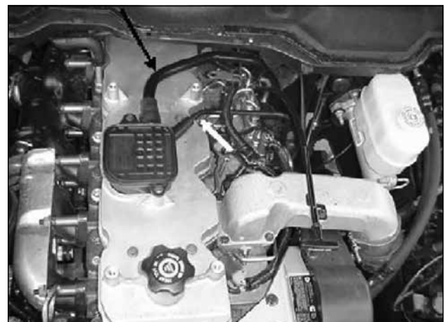
The 2003 crankcase vent system. The white arrow shows the inlet from the crankcase to the filter assembly. The black arrow points to the outlet hose that vents to atmosphere.
