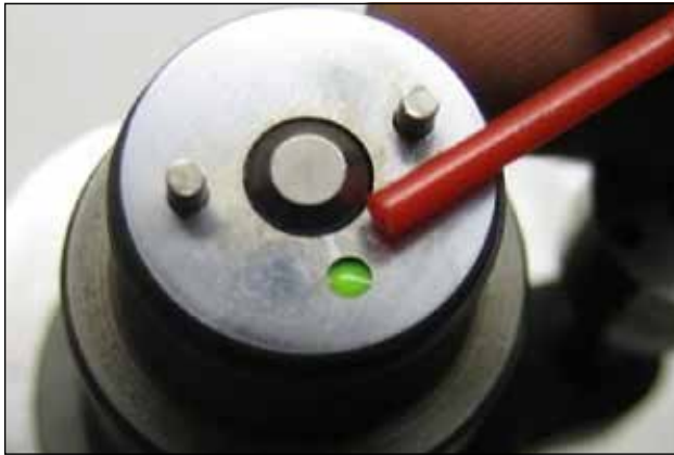
Cracked injector body.
