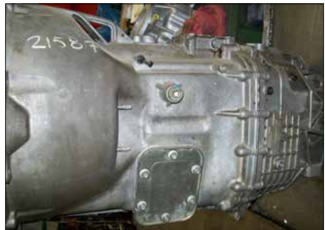
71-20 G56 two-piece transmission case.
