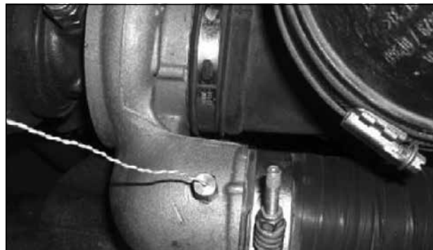
Bead-type low temperature thermocouple installed in the turbocharger compressor housing, which provided very precise and reproducible air temperature measurements at various boost pressures.
