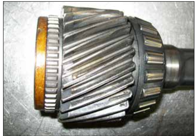
71-18 Input with wear indicating misalignment of gears.
