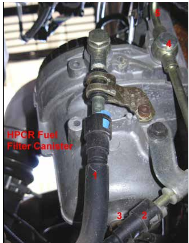
Looking at the 5.9 HPCR ('03-'07) fuel filter assembly:
