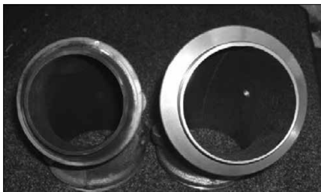
On the left is the stock 3.5" turbocharger cast elbow we removed from the test truck. Note the 3.5" downpipe opening. On the right is the cast elbow used on the '04.5-'05 trucks. Note the 4" downpipe opening.
