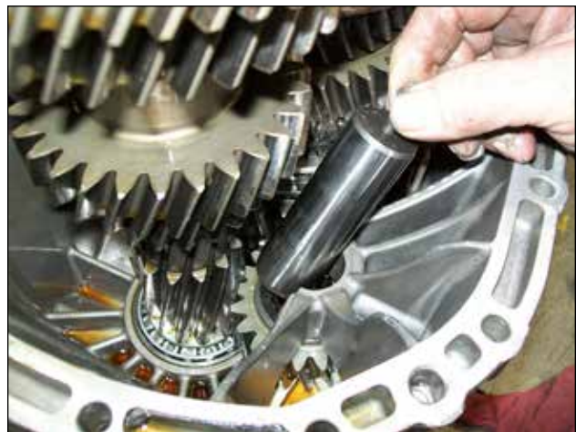
71-26 Removal of idler gear shaft.
