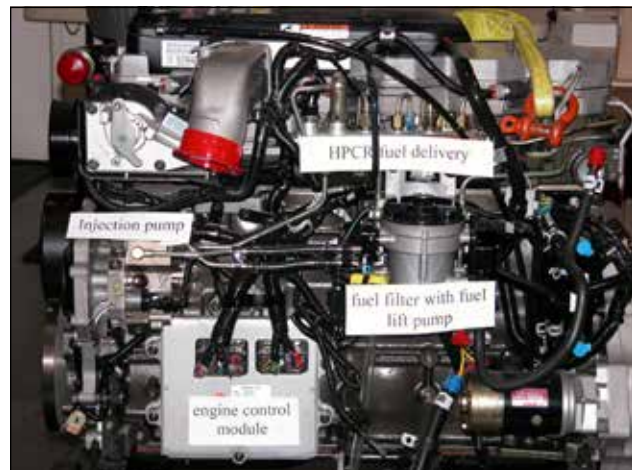
72i2. The driver's side of the 2003 HPCR Cummins engine. The injection pump, engine control module (ECM computer), HPCR fuel delivery system, and fuel filter with fuel "lift" or transfer pump are labeled.
