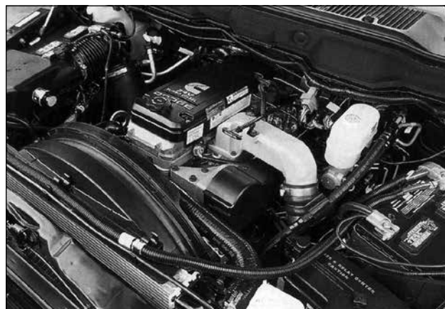
This picture is the 2004.5 engine compartment. Note the engine-mounted fan shroud and the blocker panel to the left and in front of the air cleaner box.
