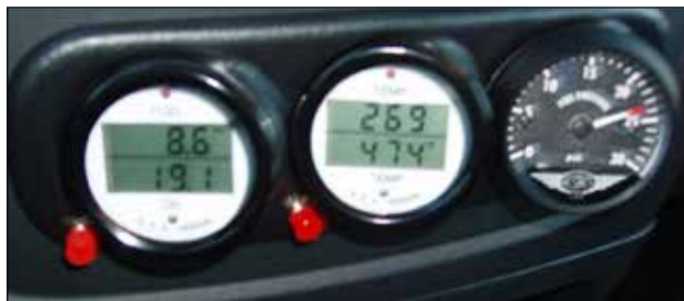
Gauge cluster installed on the test truck, capturing several parameters while the vehicle was moving. Not shown is an SPA pre-turbo EGT and boost gauge.
