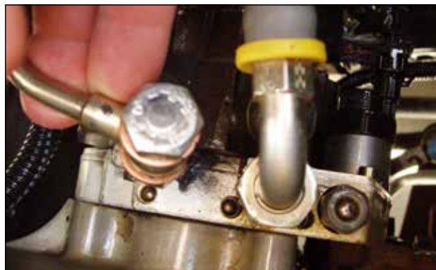
The 1/2" fuel line from the Fuel Preparator (right) attaches directly to the CP3 high pressure pump input, replacing the stock fuel line. The stock fuel line (held to the left) has been sealed with a solid bolt, 12mm copper washers, and its own banjo bolt washers. This allows easy conversion back to the stock fuel system.
