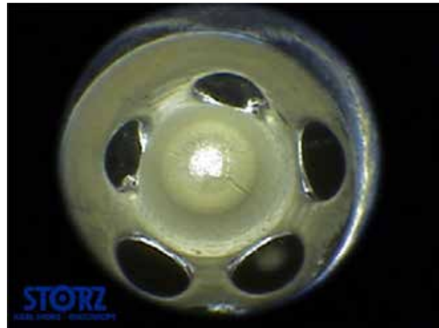
Borescope view of an extrude honed nozzle.
