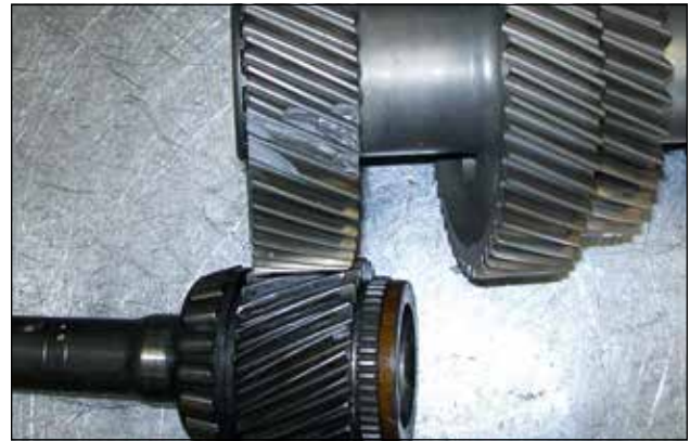
71-19 Input and cluster with broken teeth caused by poor alignment and heavy loading.
