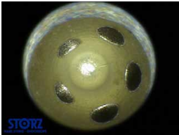
Borescope view of the inside of a 12-valve injector nozzle.
