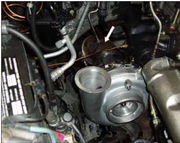
The Aurora 5000 turbocharger is shown installed with the ATS two-piece manifold. The Aurora bolts directly to the same exhaust cast elbow (see arrow) and downpipe assembly supplied for the stock truck. A post-turbo EGT probe is installed in the exhaust cast elbow. A turbocharger drive pressure line is shown going across the top of the cast elbow connecting to the manifold. A pre-turbo EGT probe is shown in the manifold right next to the heat shield.
