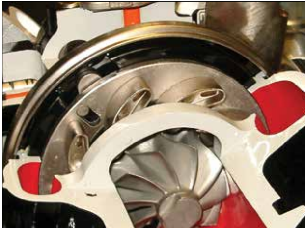
On this Ford turbocharger, the vanes are pinned to the (white) turbine housing. When the plate behind the vanes rotates, the vanes pivot around the pins like slats in a window blind. Note the slot for the crank; the plate rotates only a few degrees.
