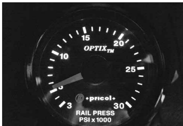
New PSI rail pressure gauge from Pricol, for the '03-'06 Turbo Diesels, showing approximately 5,000 psi at curb idle. The maximum pressure that can be measured is limited by the factory sensor and is approximately 26,500 psi. The stock truck maximum rail pressure is approximately 23,500 psi.
