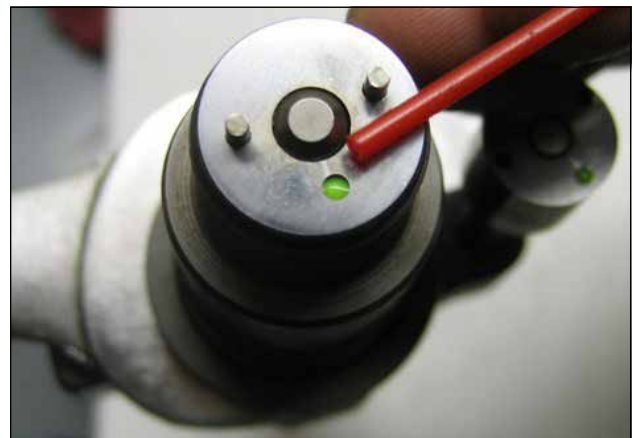
72i15. Cracked injector body.
