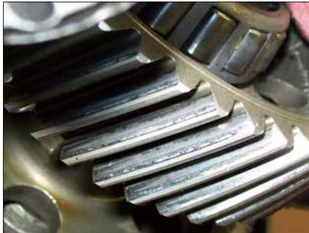
71-29 Electrolytic pitting of gear teeth.
