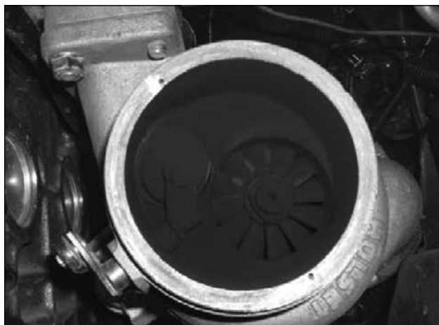
The exhaust pinwheel of the HY-35 turbocharger installed on the '03-'04 trucks. The pinwheel is inside of a 4" diameter housing that mates up directly to the exhaust elbow. The wastegate is seen directly to the left of the pinwheel. The turbocharger mounting studs and nuts are visible in the upper left.
